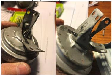
8) After the epoxy sets for a few hours, reinstall it on the distributor, put it back in the car and set your idle timing (I like a slight advance 18 degrees). You can test it to verify it is working by using the Mity Vac to pump up the capsule and monitoring the results with a timing gun: the spark should retard to 10-11 psi at about 1.0 bar of pressure. Follow the Group 9 adjustment procedure (attached at the end of this guide).
