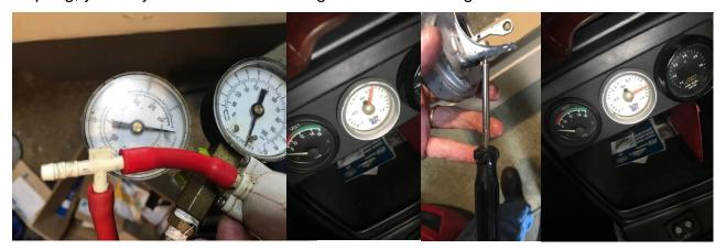
Once calibrated, you just need to put dabs of epoxy on all of the connections. I like 5-minute epoxy for this job.
